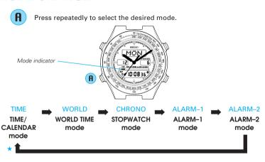
\* : When the confirmation sound is switched on, a beep sounds with each press of Button A. As a reference aide, the pitch is different when TIME/CALENDAR mode appears.
